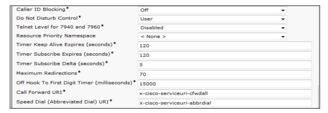
SIP Profile Configuration used by SIP trunk to Cisco UBE (Continued...)
