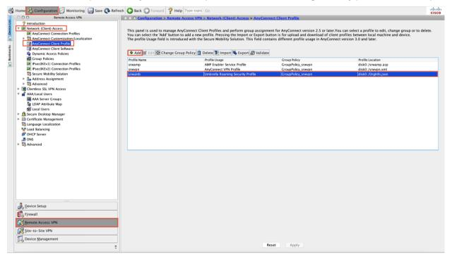
Step 3. Enable Umbrella Roaming Security Profile: Navigate to Configuration → Remote Access VPN → Network (Client) Access → Group Policy → select Group\_Policy, now ensure it has Umbrella Roaming Security Profile enabled
