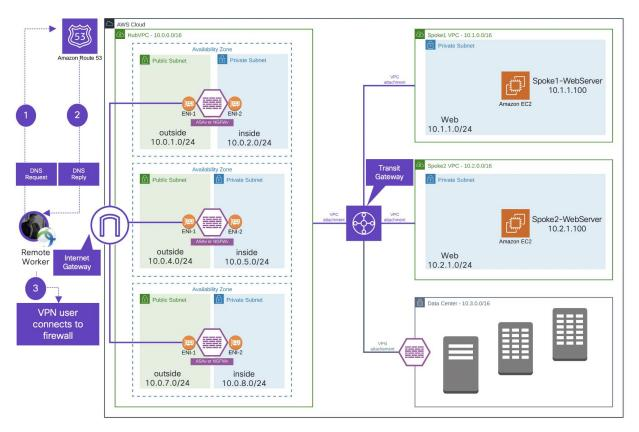
Figure 24. Secure Remote Worker architecture for multi-VPC, multi-AZ
