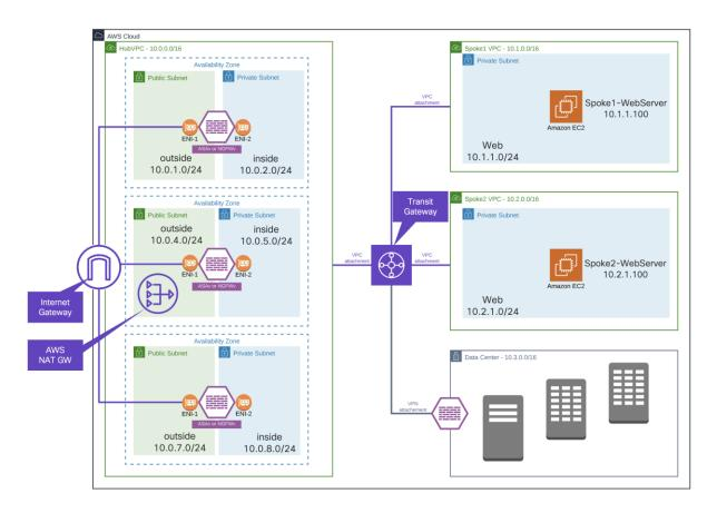
Figure 13. Outbound traffic (non-VPN traffic) uses AWS NAT gateway
