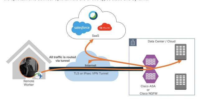
Figure 14. Remote employee accessing resources hosted in the data center (tunnel-all)
