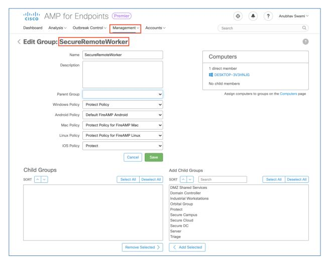
**Step 2.** Create Endpoint Group policy for RAVPN users - Create a policy for windows endpoint and attach it to the "SecureRemoteWorker" Group. Also, configure "custom detection" to block specific hash value.
