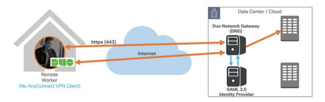
Figure 23. Non-VPN remote worker (Duo Network Gateway)
