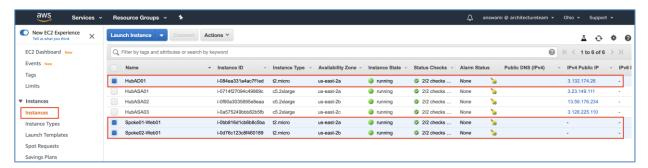
**Step 5. Deploy Cisco ASAVS** - Deploy ASAs in HubVPC - Access AWS marketplace and search Cisco ASA and deploy BYOL offering
