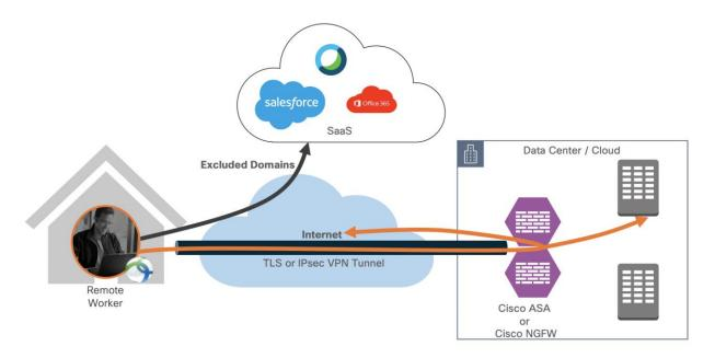
Figure 16. **Dynamic split tunnel applied (exclude traffic destined to exclude domains)**Cisco ASA natively supports a "dynamic split-tunnel" feature. On the Cisco Next-Generation firewall, the dynamic split tunnel feature is configured using Flex-Config.
