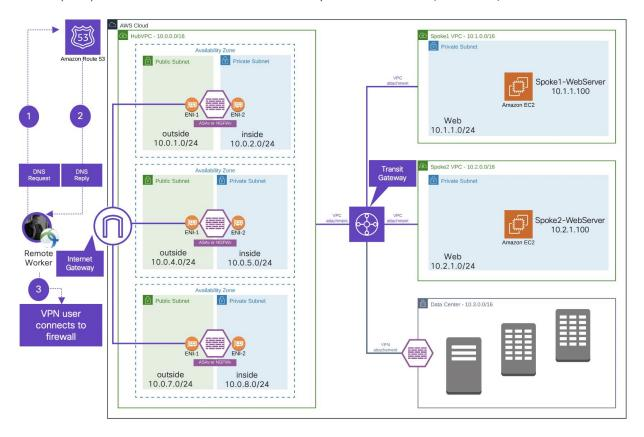
Figure 10. **Secure Remote Worker architecture for multi-VPC, multi-availability zone** The above network design has the following components and services:
