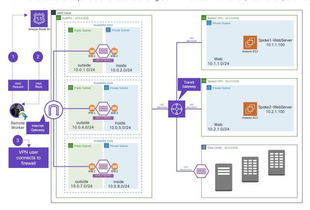
The AWS route 53 endpoint configuration ensure equal load distribution of SSL RAVPN.
