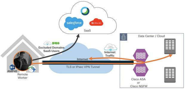
Figure 21. Remote worker is on VPN (Dynamic split tunnel – exclude domain)
