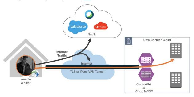
Figure 15. Traffic destined for 10.1.0.0/16 is sent through the VPN tunnel, other traffic is exempted from VPN tunnel
