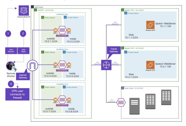
Figure 27. Components of the Cisco secure remote worker solution
