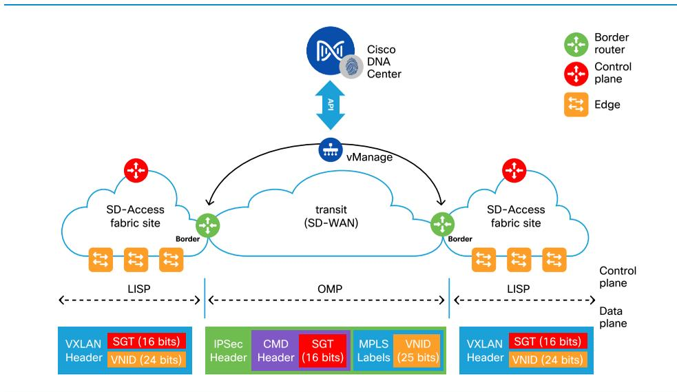
This integration achieves end-to-end secure connectivity. SD-Access identity services are critical in identifying users/things to deliver a trust-centric security layer. SD-
