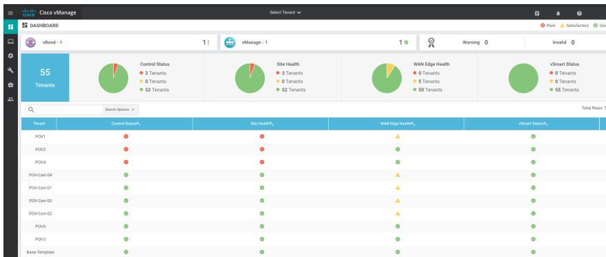
When MSPs use common WAN Edge routers to support multiple customers by leveraging VPN segmentation technology, they are able to create per-VPN tenants. In this case, a particular VPN or a set of VPNs is assigned to a specific customer, with their own configurations and monitoring dashboard environment.
