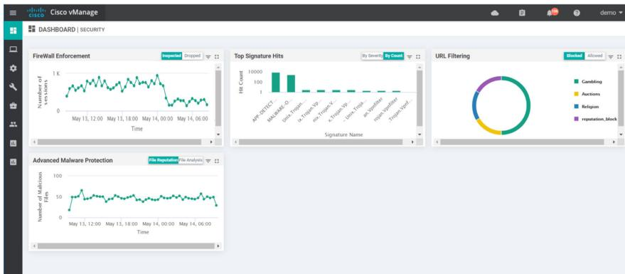
Opening up the Firewall Enforcement graph details reveals how many inspections and drops occurred over time.
