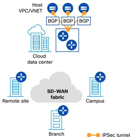
Cloud onRamp for IaaS can be used for extending SD-WAN into the public cloud. It can also be used to build a custom security stack in the public cloud.
