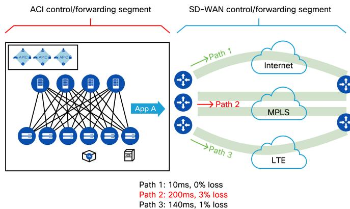
Data center to branch connectivity can be enhanced with a user-defined policy that sets the SLA for certain application traffic. Using APIs, the Cisco vManage applies the SLA policy for specific applications from APIC, and pushes it to the WAN Edge router. Once the policy is enforced, the traffic will traverse the optimal path.
