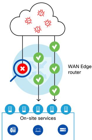
Leveraging the AMP feature, the WAN Edge router can prevent the employee from downloading a malicious file from the internet by checking the file reputation. The WAN Edge router talks to Cisco Threat Intelligence (CTI) in the background if file reputation is unknown and sandboxing is needed. Note that IPS/IDS and AMP features can also be used in the guest access use case if needed.
