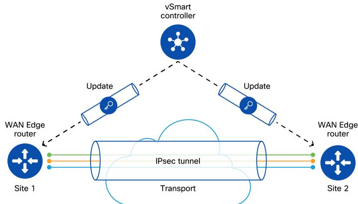
In a traditional IPsec framework, encryption keys would have been generated by the WAN Edge routers using the process known as Internet Key Exchange (IKE). One of the unique benefits of the Cisco SD-WAN architecture is how these keys are distributed via the control plane infrastructure instead. By forgoing the IKE process, Cisco WAN Edge routers can further save computational resources and scale higher.
