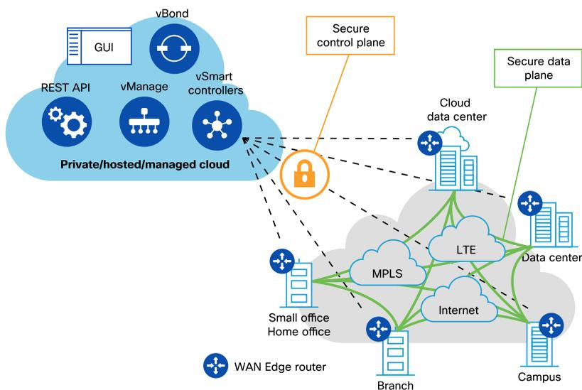
The WAN Edge routers form Internet Protocol Security (IPSec) tunnels with each other to form the SD-WAN overlay. In addition, a control channel is established between the WAN Edge routers and each of the control elements. Through this control channel, each component receives configuration, provisioning and routing information. Note that no data plane traffic is forwarded to the control infrastructure.
