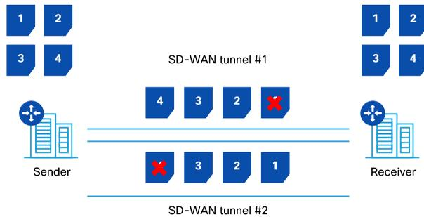
Be aware that Packet Duplication, although it increases application availability significantly, does so at the cost of increased bandwidth consumption. As a result, it should be enabled with caution.
