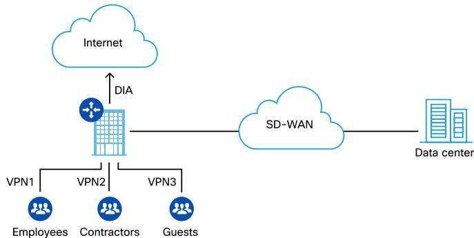
The users and branch network can be secured from the internet by implementing Cisco SD-WAN security features. Security features include application-aware firewall, intrusion protection, URL filtering, Advanced Malware Protection, and DNS security. These security features can be deployed either on the WAN Edge router itself, or as an integrated third-party security service.
