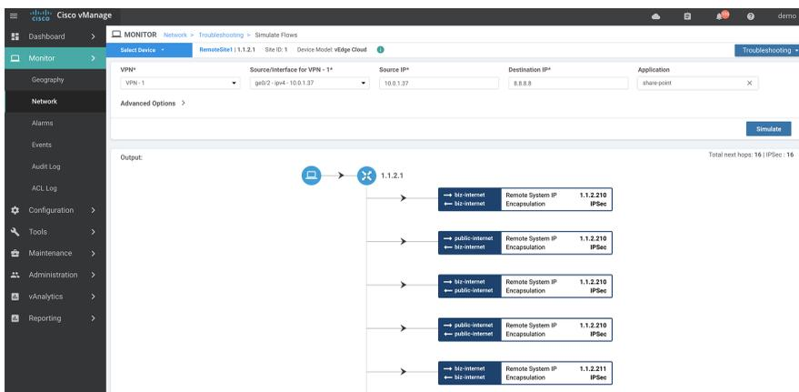
Debugs can be enabled on the router and viewed on vManage under the Troubleshooting menu as well. Log files will be streamed directly to the vManage dashboard when performing detailed troubleshooting on these devices.
