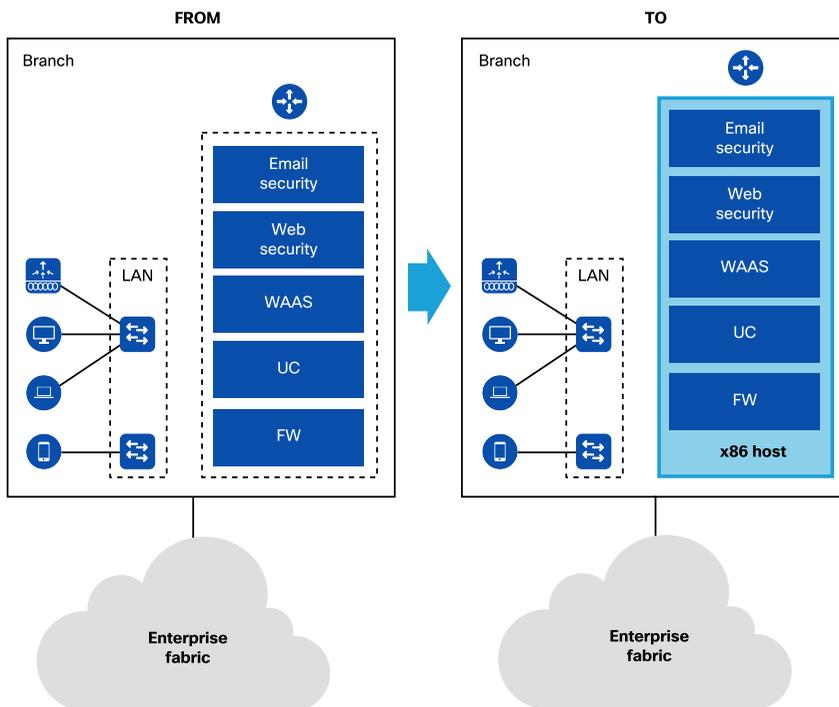
NFV solutions help with business goals by simplifying network operations to deliver new services faster. As a result, NFV allows users to reduce the cost of running services, and provides a means to generate new revenue. With NFV it is possible to run functions on general-purpose hardware, automate service delivery with orchestration, and scale easily.
