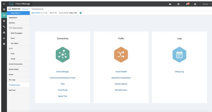
Cisco vManage allows many troubleshooting capabilities from its graphical user interface (GUI) and navigation to the individual WAN Edge router Troubleshooting sub-
