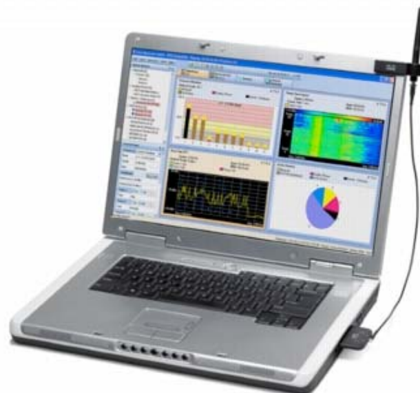
Figure 1 - Cisco's Spectrum Expert is the first spectrum analysis product designed for WLAN applications. Source: Cisco Systems.
