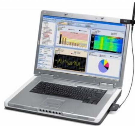
Figure 1 - Cisco's Spectrum Expert with an external antenna installed. Source: Cisco Systems.
