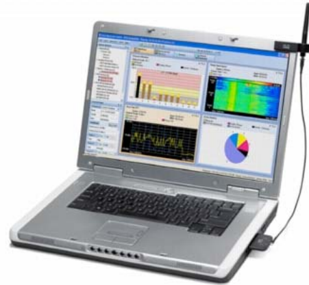
Figure 1 - Cisco's Spectrum Expert with an external antenna installed. Source: Cisco Systems.
