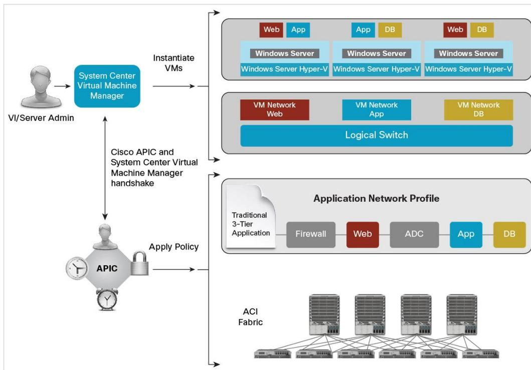
The Cisco APIC integrates with System Center Virtual Machine Manager to simplify workload connectivity. To connect Windows Server Hyper-V workloads to the Cisco ACI fabric, the virtualization administrator simply needs to associate the virtual machines with the virtual machine networks created by the Cisco APIC that appear under the logical switch in Hyper-V.
