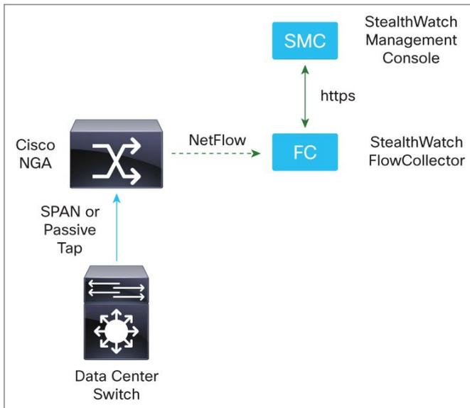
The Cisco NGA can generate and export NetFlow data using version 5, version 9 and/or IPFIX, allowing it to easily integrate with the Lancope StealthWatch System. In fact, the Lancope StealthWatch System will view the NGA just like a normal Cisco NetFlow source, such as a router.
