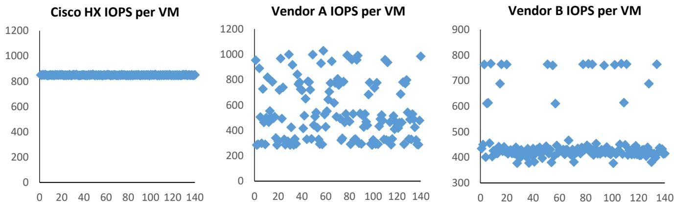
It is important to note that this variability was observed in every iteration of testing, across all block sizes and thread counts. no form of storage QoS was used during these test runs on any of the clusters. Network QoS was used for all systems.
