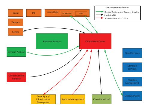
By illustrating end-point server relationships and traffic between clusters of like devices, a segment design can be validated and developed to match the client's need.
