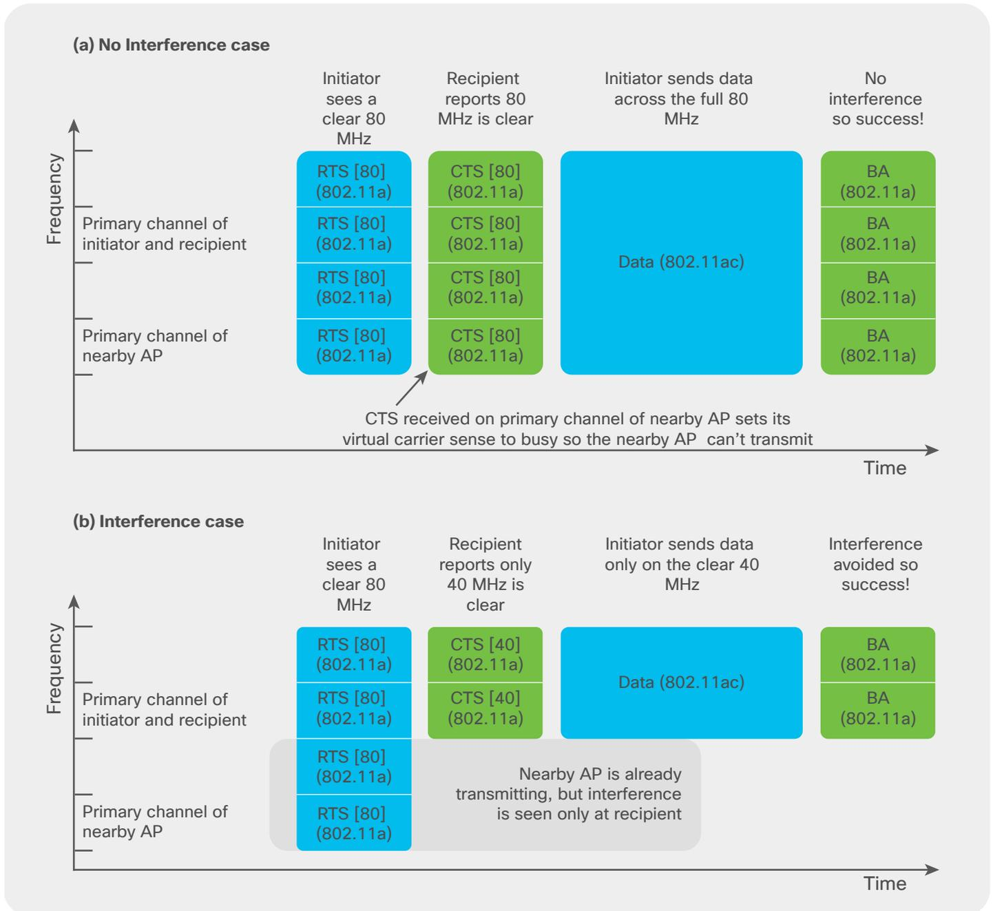
Third, the CTS is sent, like the RTS, in an 802.11a PPDU format, replicated in 20-MHz chunks across the available and useful bandwidth. Again, every nearby device receives a CTS that the device can understand on its primary channel.
