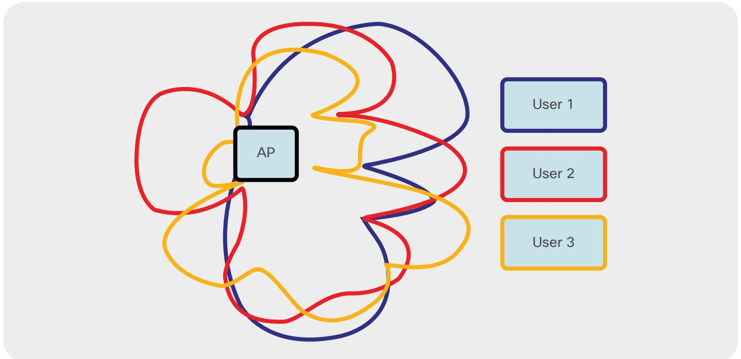
For all this to work properly, especially the deep nulls, the AP has to know the wireless channel from itself to all of the users very accurately. And since the channel changes over time, the AP has to keep measuring the channel, which adds overhead. Some APs might use the higher-overhead 802.11ac sounding protocol only, but the greatest benefit of MU-MIMO comes if the AP can minimize the number of explicit sounding exchanges, such as with the ClientLink mechanisms.
