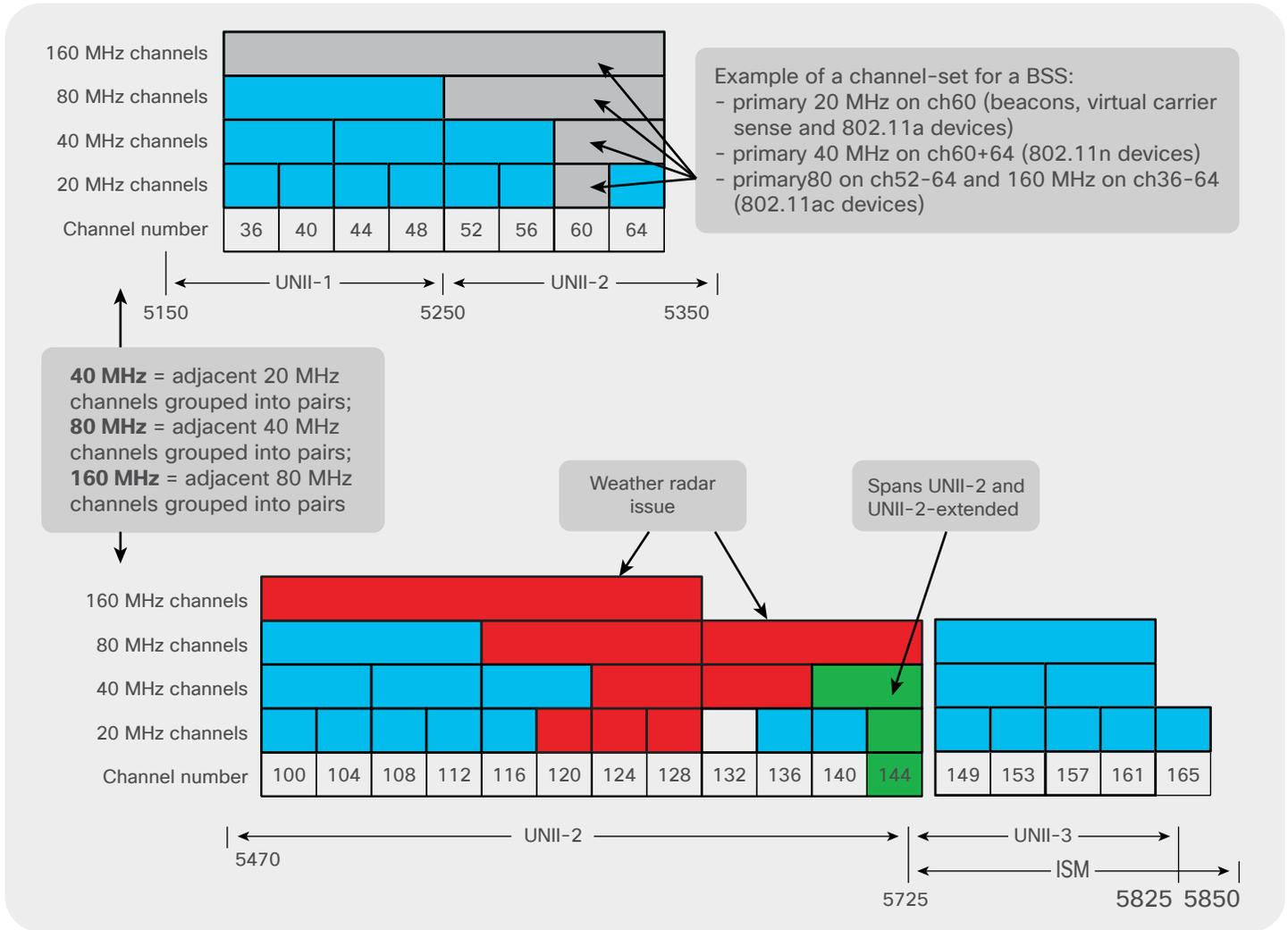
Figure 5. Example of parallel transmissions with two BSSs on the same 80 MHz but with different primary 20-MHz subchannels
