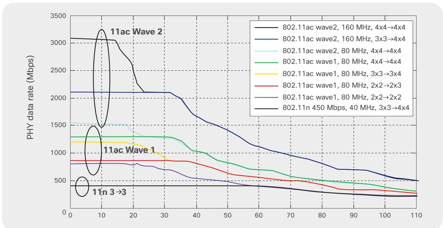
We see this improvement in [Figure 7](#), where 80-MHz links offer higher data rates close in and farther out. In Wave 1, different product configurations offer different benefits, but all are a marked step up from 802.11n. Meanwhile Wave 2, and particularly 160 MHz, potentially offers still greater speeds. However, this improvement is not immediately useful, especially in the enterprise, due to the very limited number of 160-MHz channels that are available.
