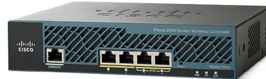
Controllers reduce overall operational expenses by simplifying network deployment, operations, and management. They allow network administrators to remotely configure and monitor several to thousands of access points in a simple and efficient way.
