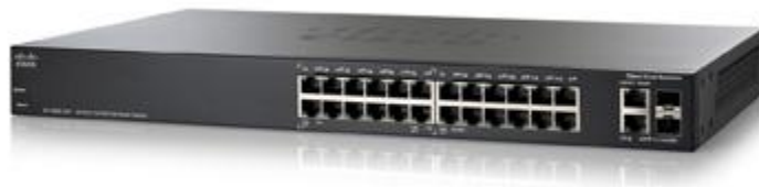
Figura 1. Smart switch 10/100 a 24 porte Cisco 200E
