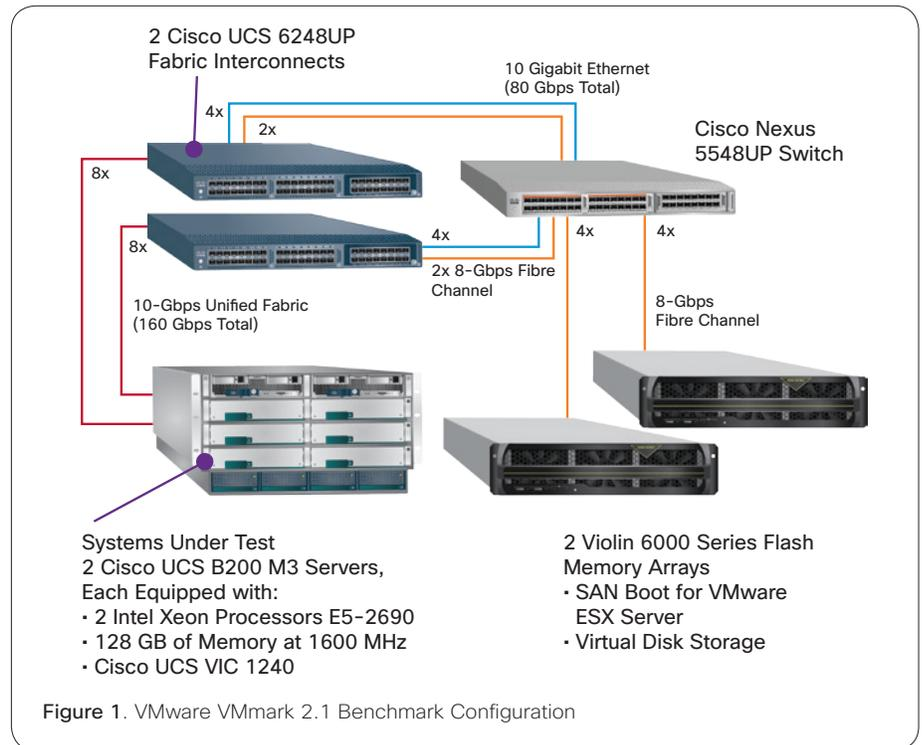
Figure 1. VMware VMmark 2.1 Benchmark Configuration
