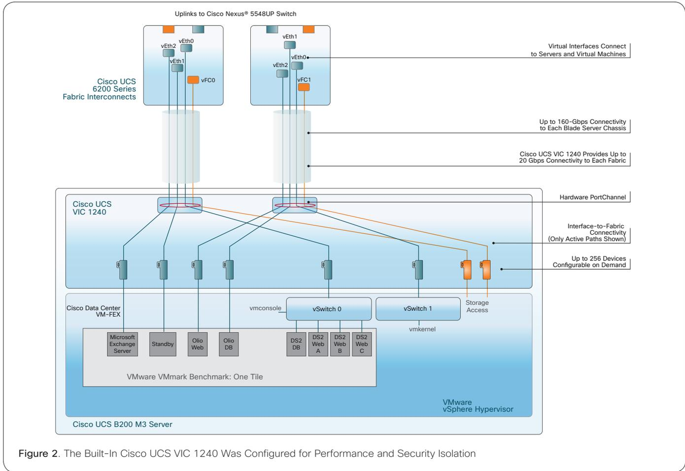
Figure 2. The Built-In Cisco UCS VIC 1240 Was Configured for Performance and Security Isolation
