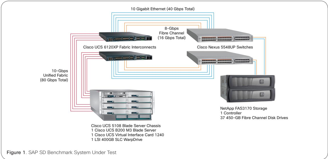
this scenario. One LSI 400-GB SLC WarpDrive, a mezzanine card deployed within the blade server, provided solid-state disk capacity for database log files that require low-latency write access.
