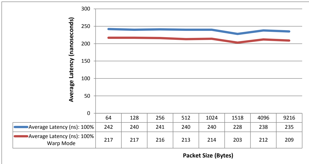
Figure 8: Layer 3 Unicast RFC 2544 Port Pair Latency Comparison: Normal Mode Compared to Warp Mode
