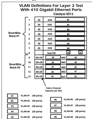
The diagram above shows how multiple Full-Mesh Traffic Groups (FMTGs) were configured and mapped to Ethernet VLANs. One Ethernet VLAN was configured for each
