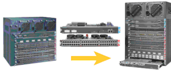
Figure 1. Catalyst 4000 Series Linecards Work in the Catalyst 4500
