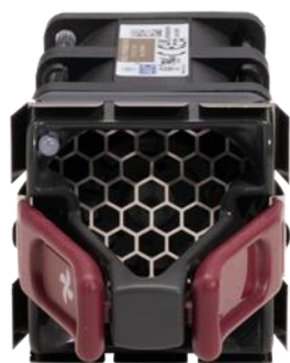
Figure 4. Field-replaceable fan units for 1RU models
