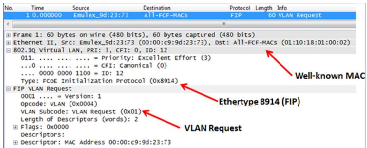
In the capture, we can see the CNA broadcast to the ALL-FCF-MAC using FIP (eth type 8914) and requesting the FCoE VLAN. The VLAN Request from the host should be received on the native VLAN. The native VLAN cannot be an FCoE VLAN.
