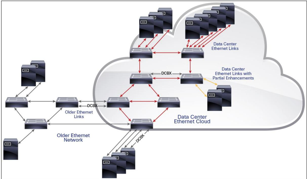
The DCBX protocol is an extension of the Link Layer Discovery Protocol (LLDP). DCBX endpoints exchange request and acknowledgment messages. For flexibility, parameters are coded in a type-length-value (TLV) format.
