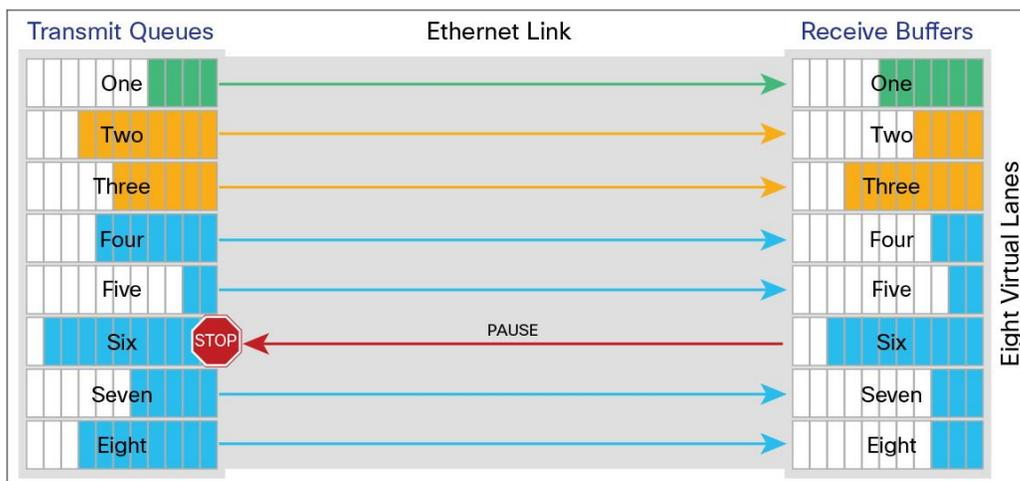
The Ethernet frames that are sent by the switch to the adapter may include the IEEE 802.1Q tag. This tag includes a field for the class of service (CoS) value used by the priority flow control (PFC). The IEEE 802.1Q tag also includes a virtual LAN (VLAN) field.
