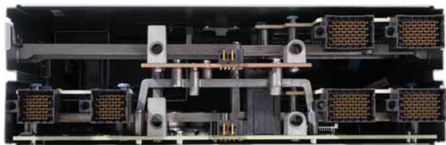
Figure 2 Front and rear views of UCS X9516 X-Fabric
