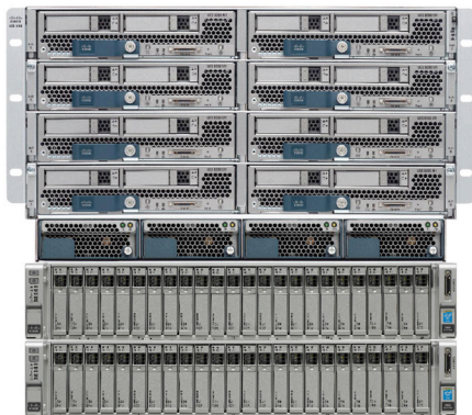
Figure 1. Cisco UCS Mini Solution for HANA with Cisco B200 Blade Servers and C240 M4 Rack Servers
