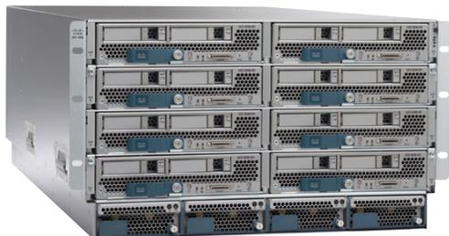
The Cisco UCS 5108 accepts between one and four 92-percent-efficient, 2500W hot-swappable power supplies that can be configured in a nonredundant, N+1 redundant, or grid-redundant design. Designed for efficiency at low utilization levels, the chassis power configuration provides sufficient headroom to support future blade servers hosting processors using up to 130W each.
