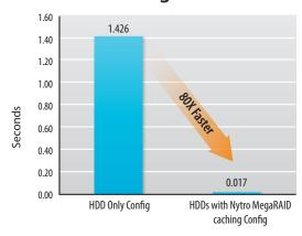
Applications that benefit from caching can also benefit from reduced rebuild time for degraded RAID arrays, even when using high-capacity HDDs. With the Nytro MegaRAID card servicing IO from the onboard flash, the backend HDDs are less burdened and can dedicate more resources to the rebuild operation.
