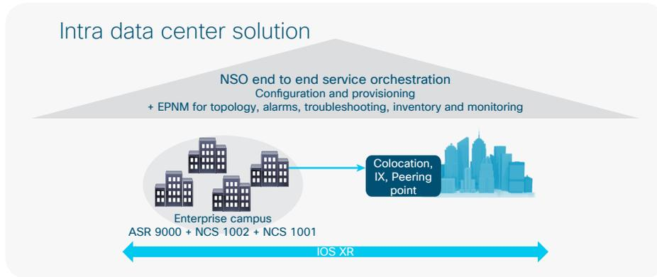
The Intra Data Center solution connects several enterprise data centers and then brings their traffic via a high-speed optical link to the closest colocation or peering point. Once the enterprise data center is located in the colocation site, it can be managed by a single management system while configuration and provisioning can be automated when Cisco Network Services Orchestrator (NSO) orchestration is deployed.
