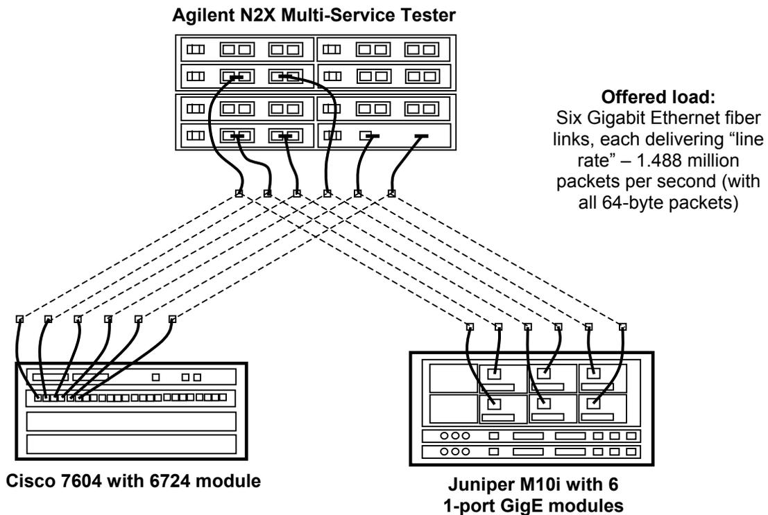
**Six fully loaded Gigabit Ethernet links.** An Agilent Technologies traffic generator, consisting of a modular chassis with dual-port, E7919B, GigE GBIC cards, and a control CPU, delivered the traffic load to the Systems Under Test (SUTs). Agilent's "N2X Packets and Protocols," version 6.4, System Release (SR1) software was used.
