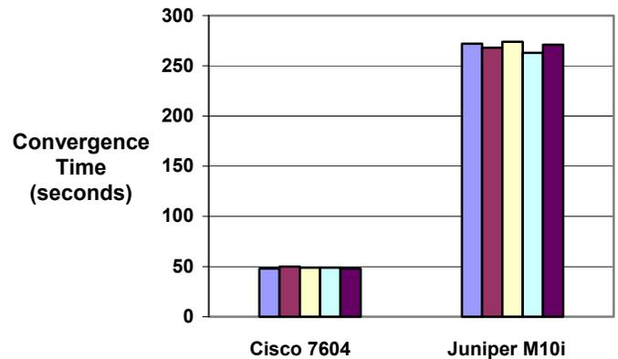
**Multicast convergence time.** The Multicast Test was run five times and the convergence time was monitored. The Cisco 7604 converged in about 50 seconds, while the Juniper M10i took over 260 seconds.
