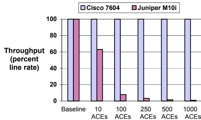
**Throughput with interface filter lists configured.** As the size of the interface filter lists was increased, the Juniper M10i throughput performance degraded. The Cisco 7604 continued to forward all packets.
