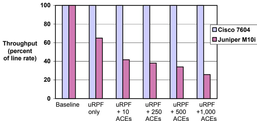
**The Cisco 7604 edge router** consistently maintains line-rate forwarding throughput even as additional services are added. When access filters and uRPF (unicast Reverse Path Forwarding) security processing are added, for example, the Juniper M10i performance degrades significantly.
