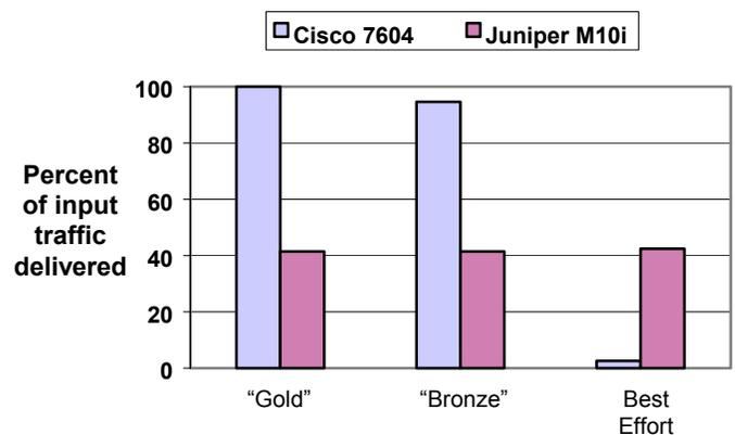
**QoS with no oversubscription.** In the baseline case, both routers faithfully delivered all high-priority traffic to the output port. However, when additional services, like uRPF or ACLs (with only 10 ACEs) are added to the configuration, the Juniper M10i begins dropping high-priority traffic even when the links are not congested.
