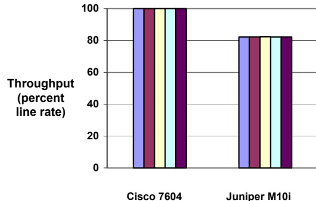
**Multicast throughput.** The Multicast Test was run five times and overall throughput was closely monitored. The Cisco 7604 forwarded 100% of the traffic after the test reached steady state, while the Juniper forwarded about 82%.
