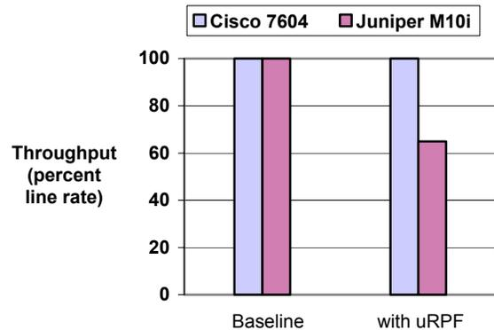
**Throughput with uRPF.** When uRPF (unicast Reverse Path Forwarding) is configured on the routers, Juniper's throughput drops to below 65% of line rate. The Cisco 7604 continues to forward at line rate.
