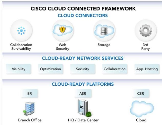
**Cloud-Ready Platforms:** The Cloud-Ready Platforms are Cisco’s Integrated Services Router or ISR G2 for branch offices, Aggregation Services Router or ASR 1000 for headquarters/data center plus internet access, and the new CSR or Cloud Services Router for the cloud. The CSR platform is a virtualized version of the ASR IOS XE image. It will eliminate most traffic hairpinning/backhauling by delivering secure connectivity directly to the cloud from the remote sites.
