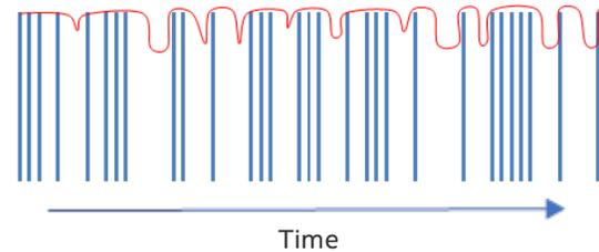
As shown by the red line, components have less time between DMA calls to reach and stay in lower power.
