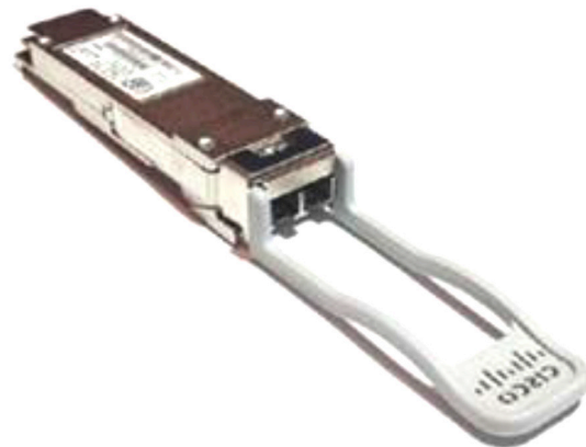
Figure 1. Cisco QSFP BiDi Transceiver (QSFP-40G-SR-BD)
