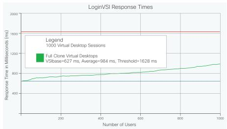
Figure 1 Average Response Time Results for Login VSI 4.1 Knowledge Worker Workload Running in Benchmark Mode
