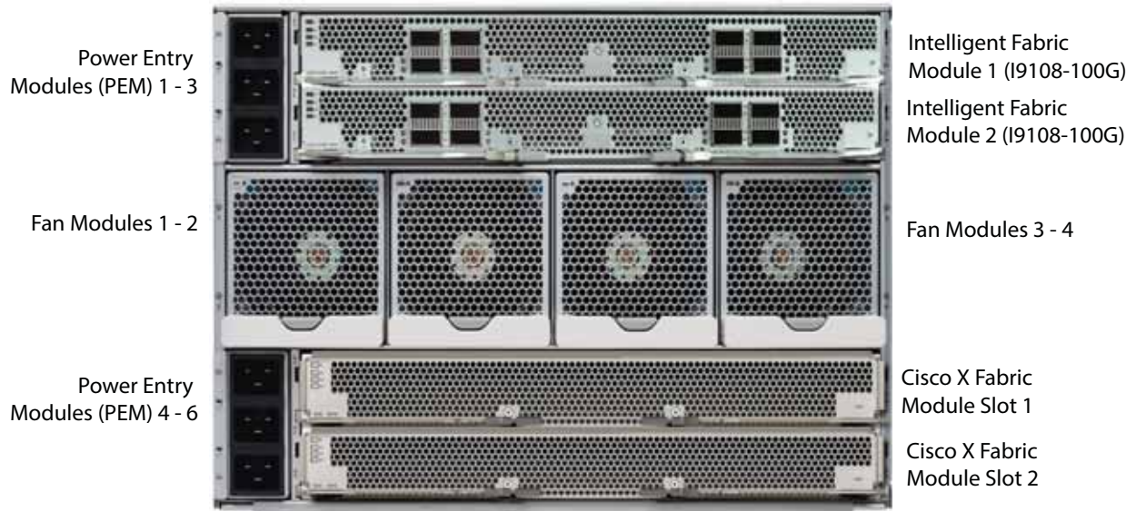
Figure 3 Cisco UCS X9508 chassis Rear View with UCSX-I9108-100G (top) and 2 Fabric Module Slots (bottom)
