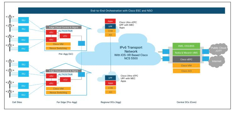
The architecture enables a lean cell site for RMN comprising the antenna and remote radio head. It supports coordinated radio processing to increase spectral efficiency, facilitates scale out, and exposes open APIs that enable multiple vendors to participate and contribute.
