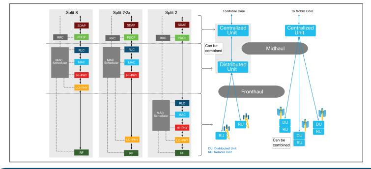
Figure 1. Radio signal processing stack.
