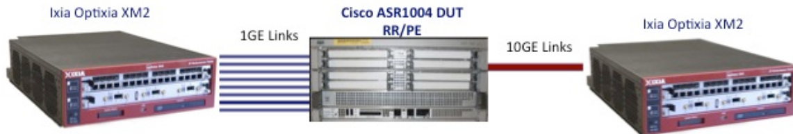
Figure 1: Cisco ASR 1004 Control Plane and provider-edge testing
