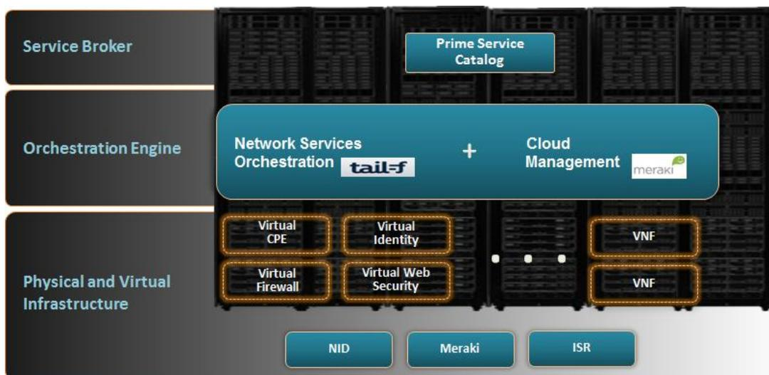
**Figure 1 – Virtual Managed Services Using Cisco ESP**
