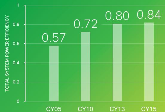
\* Total internal system power conversion and distribution from plug to ASIC; covers the complete internal power system conversion.
