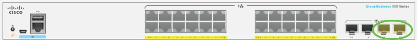
Stacking port Network port Active stack connection
