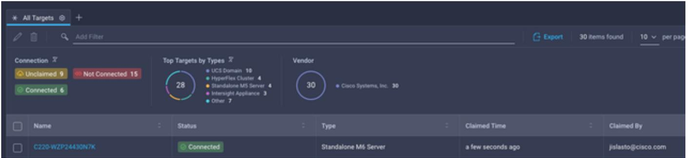
The screenshot shows the 'All Targets' page in Intersight. It includes a search bar, an 'Export' button, and a table of targets. The table has columns for Name, Status, Type, Claimed Time, and Claimed By. One target is listed: C220-WZP24430N7K, which is 'Connected' and is a 'Standalone M6 Server'.
