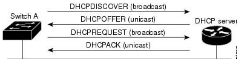
Figure 106: DHCP Client and Server Message Exchange
