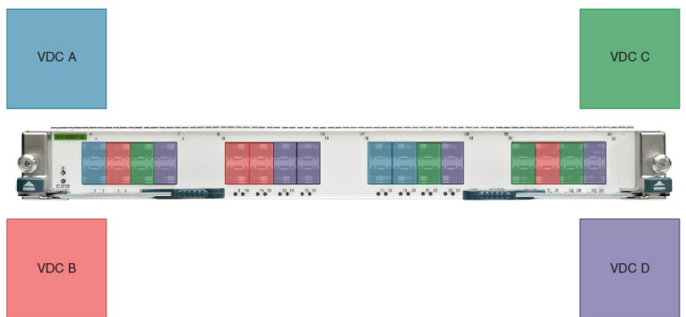
Figure 4: Example Interface Allocation for Port Groups on a Cisco 7000 Series 10-Gbps Ethernet Module (N7K-F132XP-15)
