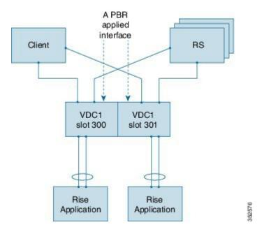
• Each appliance is connected to a different Cisco Nexus switch and each switch is in virtual port channel (vPC) mode through a peer link.
