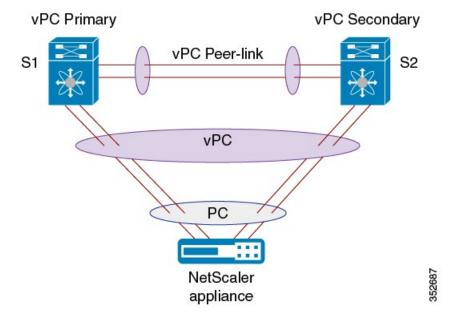
In a vPC indirect mode deployment, the service appliance is indirectly attached to a Cisco Nexus vPC peer through a Layer 2 network. The following figure shows the topology for a vPC indirect mode deployment.
