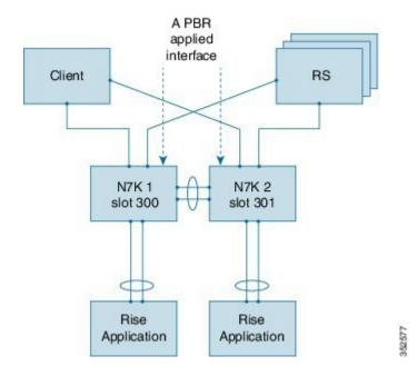
• Two appliances are each connected to a different VDC in the same Cisco Nexus Series switch.
