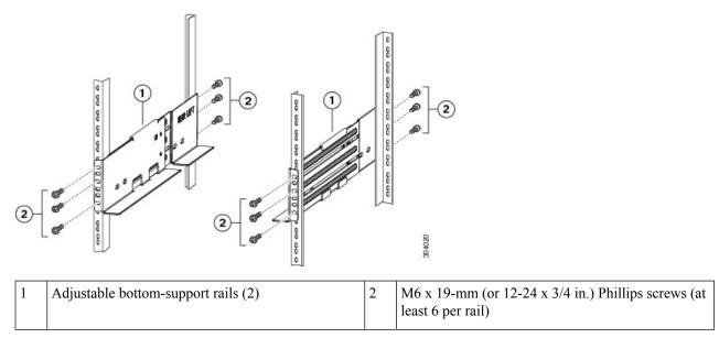
**Note** Use at least three screws on each end of each bottom-support rail.
