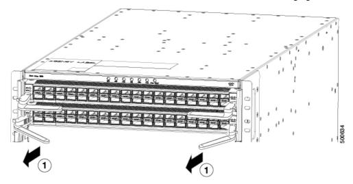
Pull both levers to remove the line card from the chassis.
