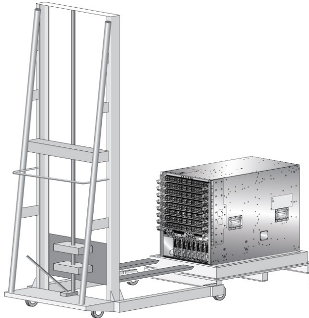
Figure 8: Align the Lifting Device in Front of the Chassis on the Pallet
