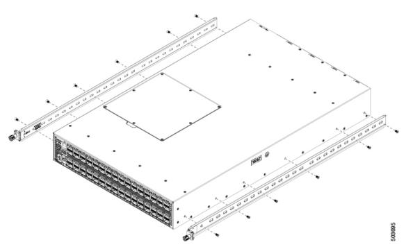
**Step 2** Install the two outer rails to the front posts of the rack by aligning the rails to the post holes, as shown in the following illustration:
