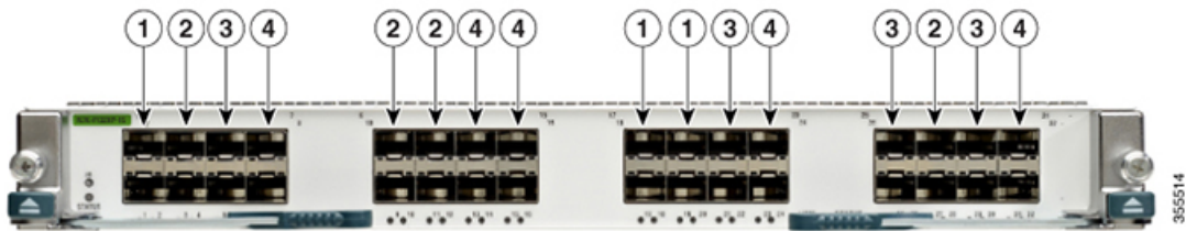
Figure 14: Example Interface Allocation for Port Groups on a Cisco 7000 Series 10-Gbps Ethernet Module (N7K-F132XP-15)
