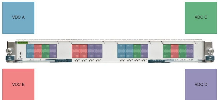
Figure 4: Example Interface Allocation for Port Groups on a Cisco 7000 Series 10-Gbps Ethernet Module (N7K-F132XP-15)
