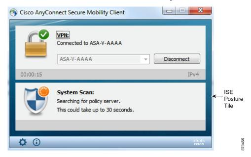
A network change starts the discovery phase. With AnyConnect ISE Posture, if the default route of the primary interface is changed, it brings the agent back to the discovery process. For example, when WiFi and the primary LAN are connected, the agent restarts discovery. Likewise, if WiFi and the primary LAN are connected but then WiFi becomes disconnected, the agent will not restart discovery.
