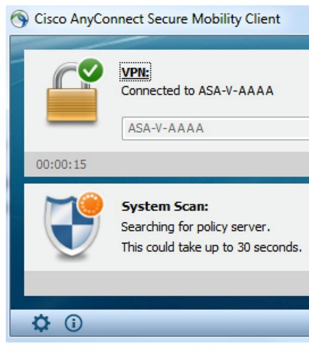
A network change starts the discovery phase. With AnyConnect ISE Posture, if the default route of the primary interface is changed, it brings the agent back to the discovery process. For example, when Wi-Fi and the primary LAN are connected, the agent restarts discovery. Likewise, if Wi-Fi and the primary LAN are connected but then Wi-Fi becomes disconnected, the agent will not restart discovery.
