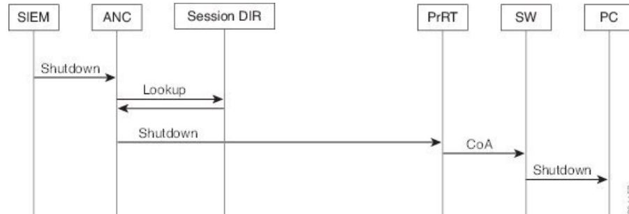
Figure 11: ANC Shutdown Flow
