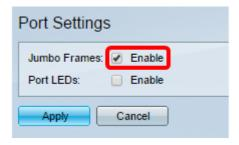
Step 3. (Optional) Check the **Enable** check box for Port LEDs in order to save power consumed by device LEDs. This feature allows you to disable the LEDs when they are not required, and to enable them if they are needed such as in situations like debugging and connecting devices. This feature is enabled by default.
