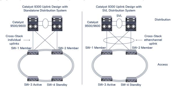
**Figure 21.**Cisco Catalyst 9300 Series StackWise-1T/480/320 uplink design best practices
