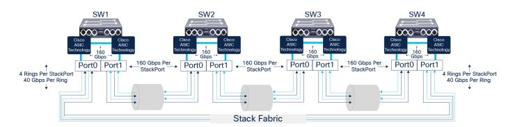
**Figure 9.**Cisco 9300L/9300LM Stackwise-320 internal forwarding architecture (Fixed Uplink Models)
