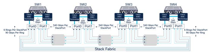
**Figure 7.**Cisco Catalyst 9300X StackWise-1T internal forwarding architecture (Modular Uplink Models)
