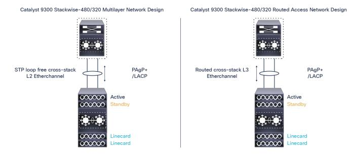
**Figure 22.**Cisco Catalyst 9300 Series cross-stack EtherChannel design
