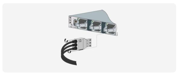
**Figure 3.**Stack cable and stack cable slot for 9300 modular uplink models (C9300 and C9300X)
