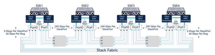
**Figure 8.**Cisco Catalyst 9300 StackWise-480 internal forwarding architecture (Modular Uplink Models)
