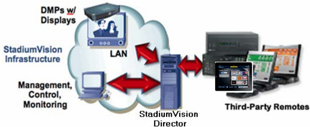
Figure 9. Local TV Control Using a Third-Party Touch Panel or User Control API Device
