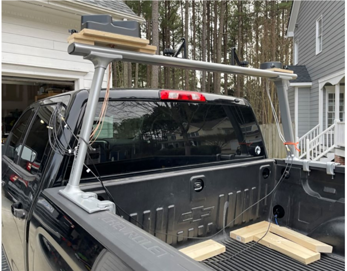
Figure 33. Antennas mounted on test vehicle
